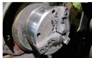
Improved runout accuracy with the chuck replaced
